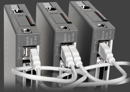
XENAX® Xvi 75V8 servo controller with Master-Slave operation, predestined for Pick & Place
