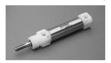
The Bimba PCE cylinder has stainless steel body, stainless steel rod and Delrin<sup>®</sup> end caps. It is ideal for applications or operating environments that require exposure to moisture, lubricants and specific solvents.
