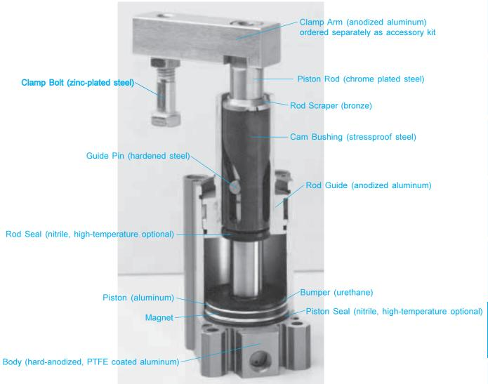
The Guide Pin rides in the Cam Bushing. The bottom portion of stroke is linear travel. As the cylinder extends, the pin follows the groove and creates 90 degrees of rotary motion.
