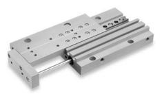
The LPA actuator was developed for applications that require precise load guiding, with ultra-tight space constraints. This actuator minimizes thickness with a linear recirculating ball rail located next to the bore.
