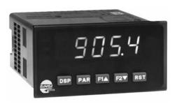
The DPM controller is ideal for measuring and gauging applications. The measurement repeatability, when combined with the PFC, is 0.001 inch per inch of stroke. The DPM supplies the PFC with a very accurate excitation voltage and has a 16 bit A/D converter. The DPM/PFC combination can be used as a Go/No Go gauge for in process quality control, among other things. A typical application follows:
