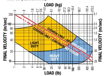
NOTE: If final (impact) velocity cannot be calculated directly, a reasonable guideline to use is 2X average velocity.
