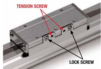
3. Tighten tension screws by turning them clockwise until the carrier is just tight enough so that no side-to-side rocking motion is present and it can easily be moved by hand over the entire stroke length with no hesitation. Very little torque on the screws is required to obtain this condition.
