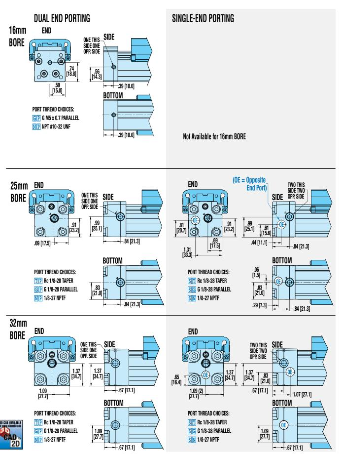
Dimensions in inches [brackets indicate dimensions in millimeters]
