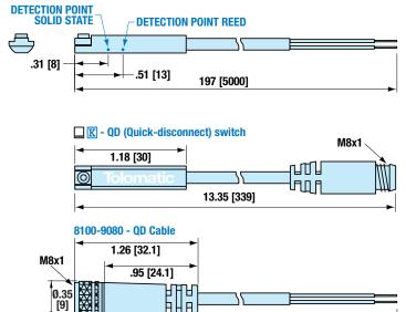
Dimensions in inches [brackets indicate dimensions in millimeters]
