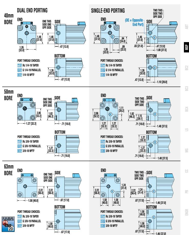
Dimensions in inches [brackets indicate dimensions in millimeters]
