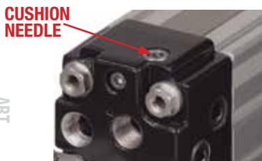
Adjust the cushion needle in the cylinder heads carefully to obtain proper deceleration for your particular application. Proper cushion needle adjustment is achieved when the carrier reaches the end of travel at a velocity approaching
