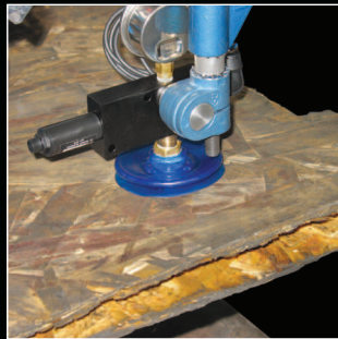
Robotic palletizing application: worn wooden slip sheet handling
