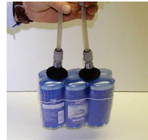
VP10 with bellows cups – pick and place deodorant packages for packing application.
