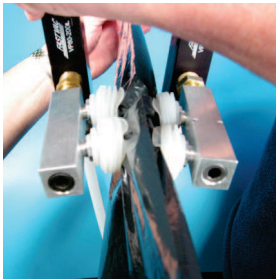
▲ Bag Opening Sequence: Two VP80 pumps w/multi-bellows cups. Bag closed.
