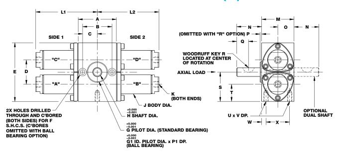
Note: Body retainer on 2" bore has 4 corners. L1/L2 dimensions shown in chart on page 4.8.
