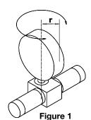
Thin Disc (mounted on side through center)
