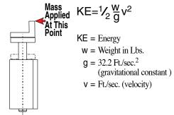
In applications such as conveyor stops impact loading may be a factor. The table below gives the maximum KE energy for each of the PB2 models. Use the above equation to determine the KE for your application. Your result should not exceed the maximum KE for the PB2 model you select.
