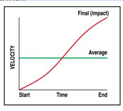
final (or impact) velocity. Rodless cylinders accelerate and decelerate at each end of the stroke. Therefore this acceleration must be considered (see diagram).
