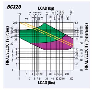
NOTE: If final (or impact) velocity cannot be calculated directly, a reasonable guideline to use is 2 x average velocity.
