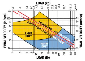
NOTE: If final (impact) velocity cannot be calculated directly, a reasonable guideline to use is 2X average velocity.
