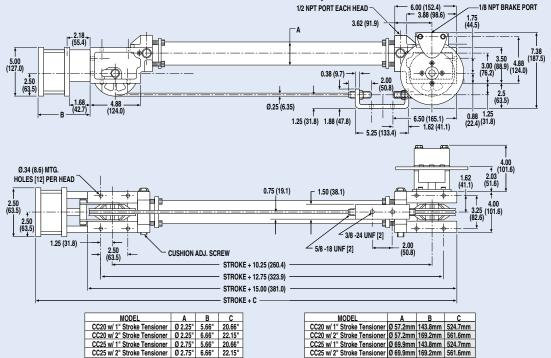
Dimensions in inches, in parentheses ( ) dimensions in millimeters
