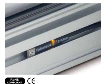
MX products offer a large number of sensing choices. There are 12 switch choices: reed, solid state PNP (sourcing) or solid state NPN (sinking); in normally open or normally closed; with flying leads or quick-disconnects.
