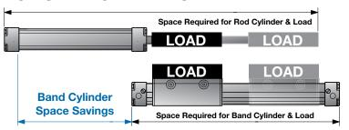
**Consider this:** A rodless band cylinder contains its stroke within the cylinder itself. A 2" bore cylinder with a 24" stroke can provide a 43% space savings when compared to an equivalently sized tie rod cylinder. In addition, the load is supported throughout the entire stroke so there is minimal bearing wear and load deflection when compared to rod style cylinders.
