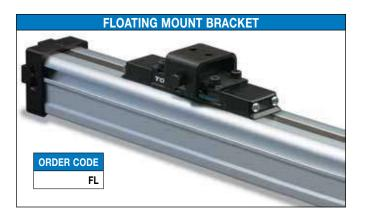
For applications where a BC4 band cylinder is moving a load that is externally guided and supported. An externally guided load, not parallel to the BC4 band cylinder may result in cylinder binding. The floating mount bracket compensates for nonparallelism between the cylinder and the external guide.
