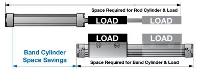
Consider this: A rodless band cylinder contains its stroke within the cylinder itself. A 2" bore cylinder with a 24" stroke can provide a 43% space savings when compared to an equivalently sized rod cylinder. In addition, the load is supported throughout the entire stroke so there is minimal load deflection when compared to rod style cylinders.
