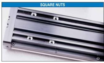
\*NOTE: Four square nuts are provided with each linear slide for base mounting. Additionally 2 square nuts are provided for 30" of stroke and 2 for every 20" of stroke thereafter.
