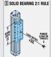
For applications using [S] solid bearings, binding or interrupted motion may occur if the load offset is equal to or greater than twice the bearing length (1X). LOAD OFFSET is defined as: the distance from the applied force (or the load center of gravity) to the centerline of the carrier.
