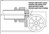
Proof-loading and pretensioning involve removing the two types of stretch in the cable by adjusting the clevis terminal lock nuts.
