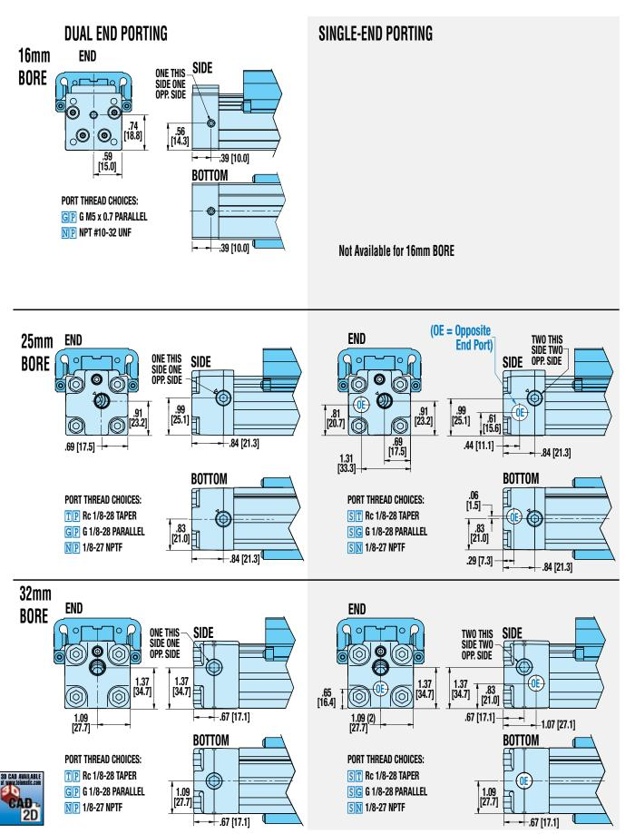
Dimensions in inches [brackets indicate dimensions in millimeters]
