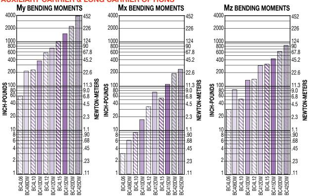
\*Auxiliary carrier bending moments indicated are at minimum center to center distance. Additional My + Mz load capacity can be obtained by increasing "D" dimension. Refer to auxiliary carrier data on page BC4\_20.
