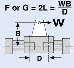
**L** should be below curve for the corresponding slide on the "Load vs. Stroke" chart (for sintered bronze or linear bearings - Mag Coupled Slides).
