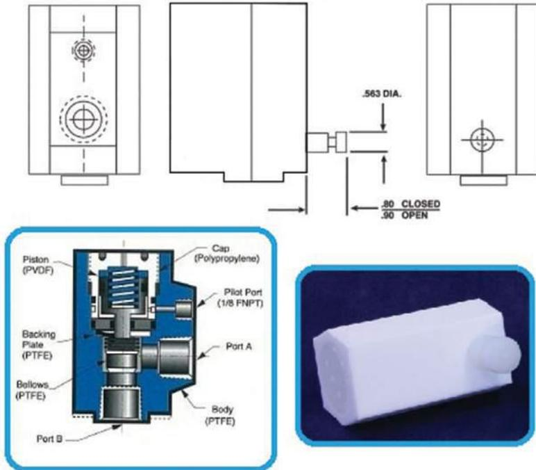
This style TP Valve offer a continuous metered flow path to reduce the potential of chemical and bacteria build-up.
