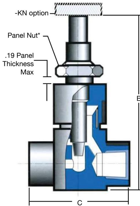
\*Stem Style Adjustment Knob supplied with the panel mount version. This is the standard Metering Valve configuration.
