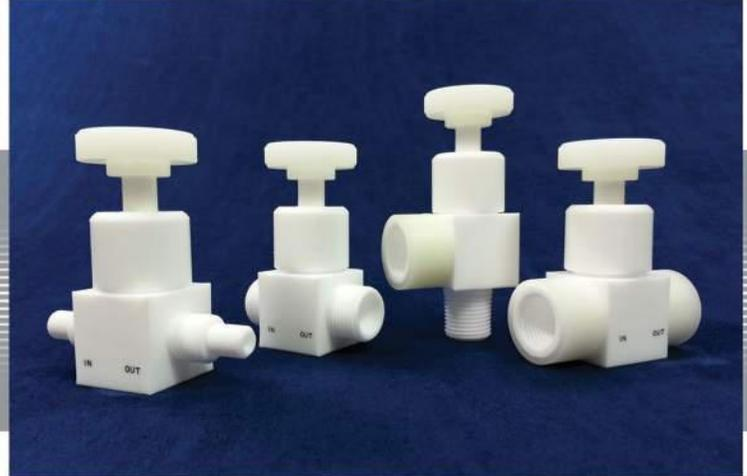
**IPS Metering Valve (MV)** use a tapered plug-stem to give a fine adjustment to the flow in addition to a full, open, or positive shutoff position.
