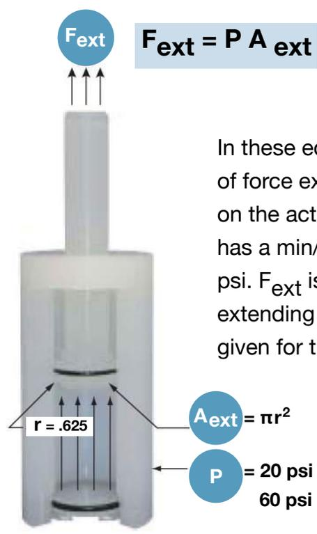
In these equations, F equals the amount of force exerted by the piston depending on the actuation pressure. The Air Cylinder has a min/max actuation pressure of 20-60 psi.  $F_{ext}$  is the variable given for the force extending the piston.  $F_{ret}$  is the variable given for the force retracting the piston.
