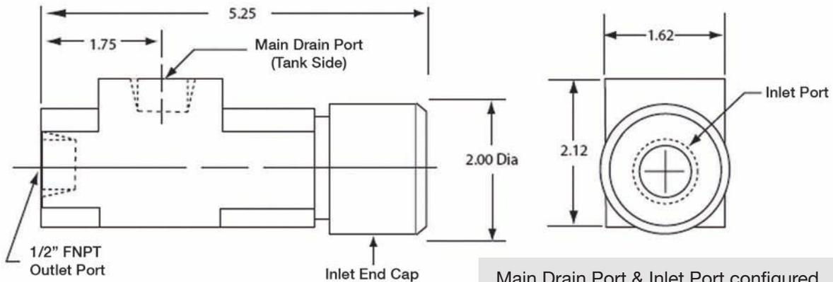
Main Drain Port & Inlet Port configured to match (see below)
