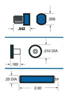
These small High-Purity PTFE Fittings are design to mate with 1/32", 2/32" and 3/32" I.D. precision tube.
