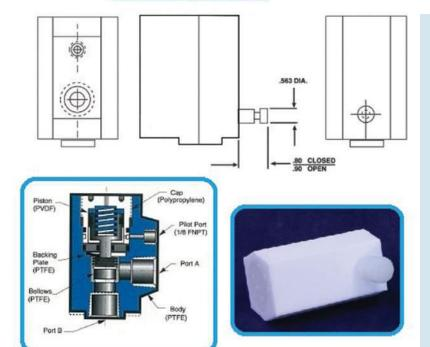
This style TP Valve offer a continuous metered flow path to reduce the potential of chemical and bacteria build-up.
