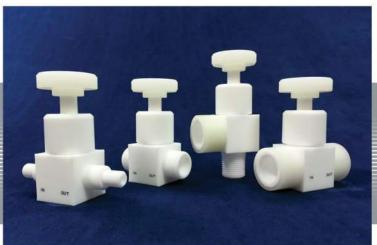
**IPS Metering Valve (MV)** use a tapered plug-stem to give a fine adjustment to the flow in addition to a full, open, or positive shutoff postition.
