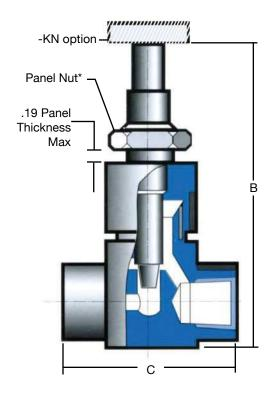
\*Stem Style Adjustment Knob supplied with the panel mount version. This is the standard Metering Valve configuration.
